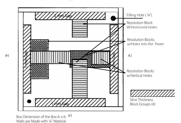
Figure 1-3. Resolution Sections in Three Imaging Planes
